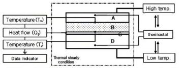
A: high temperature plate B: test specimen C: heat flow meter D: low temperature plate
