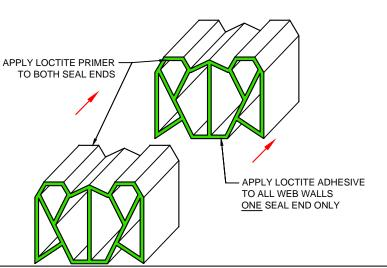
STEP 2 - Adjoin ends of seal together by applying Loctite Primer to both ends and Loctite Adhesive to only one of the ends to be joined. Hold ends together for approximately 15 seconds.
