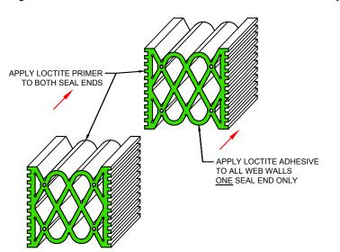
**STEP 2** - Adjoin ends of seal together by applying **Loctite Primer** to both ends and **Loctite Adhesive** to only one of the ends to be joined. Hold ends together for approximately 15 seconds.
