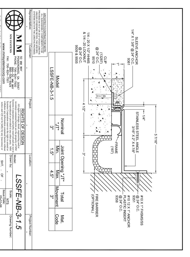
For Spec-Data, Installation Guides, or movement requirements, contact MMSC
