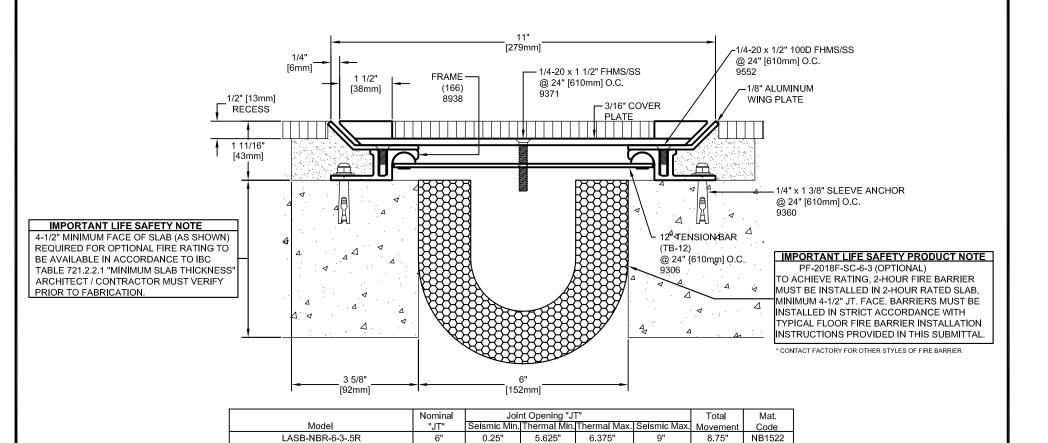
LASB-NBR-6-3-.5R w/ PF-2018F-SC-6-3 SIGHT LINE MATCHES LASB-NBR-6-1.5-.5R
