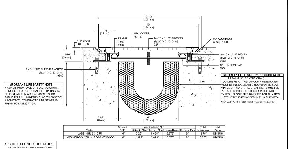
ALL SUBASSEMBLY COMPONENTS TO BE PROVIDED IN 10'-0" OR 20'-0" STOCK LENGTHS UNLESS OTHERWISE NOTED. THE SPECIFIC SYSTEMS DICTATE THE LENGTHS PROVIDED.
